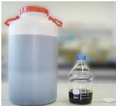
Figure 3: About 800 mL of concentrate or 600 g of dry solids can be produced from 20 L of nitrified urine.
